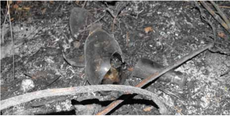
Bottles or broken glass may contain traces of accelerants such as petrol or paraffin
