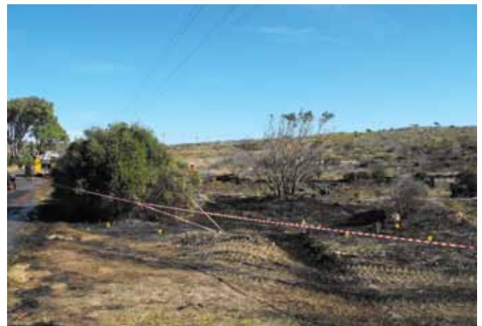
Where possible, use barrier tape to cordon off the general origin of the fire to prevent damage to evidence
